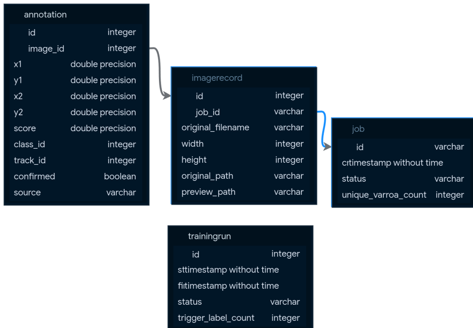
Figure 4.4: PostgreSQL database schema of the backend service.
